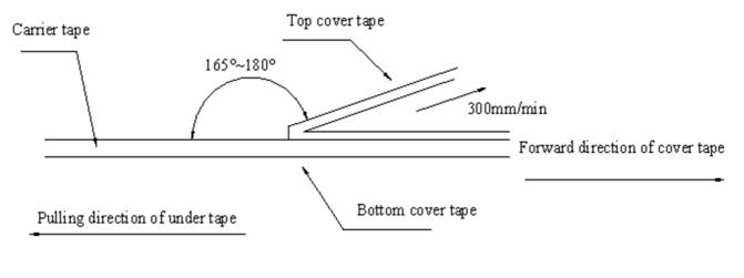
\*\*\* In the case, the cover tape is pulled off under the above conditions, the cover tape adhesion strength should be 10.2g~71.4g Plastic tape:10.2g~71.4g
