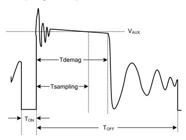
Figure 2. Auxiliary voltage waveform
