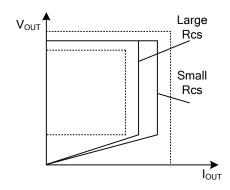
Figure 3. Adjustable output power by changing R<sub>CS</sub>
