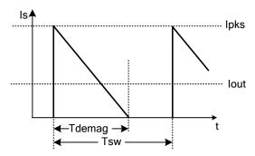
Figure 4. Secondary current waveform
