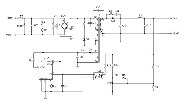
Fig.8 UTC UCS1655S Typical Application Circuit
