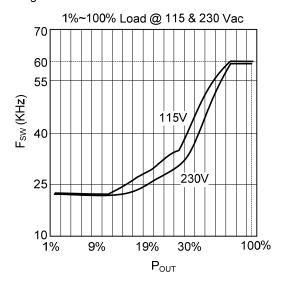
Fig.4 The relation curve between  $f_{\text{SW}}$  and relative output power  $P_{\text{OUT}}$
