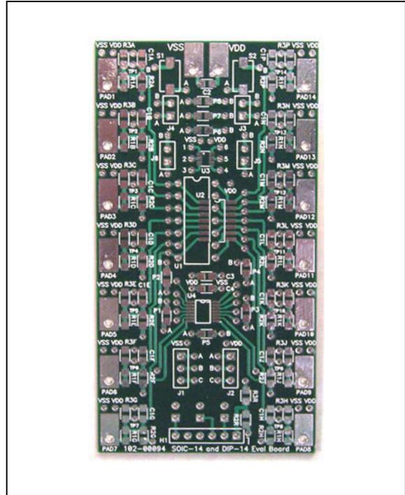
**FIGURE 8-2:** SOIC-14 Evaluation Board (Microchip Part Number SOIC14EV).
