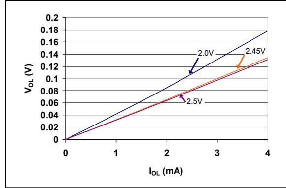
**FIGURE 2-18:**  $V_{OL}$  vs.  $I_{OL}$
