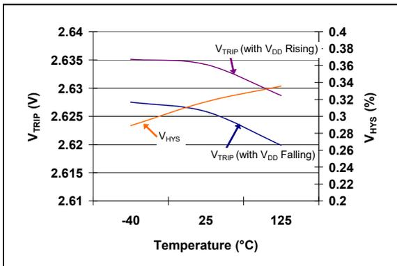
**FIGURE 2-15:**  $V_{TRIP}$  and  $V_{HYS}$  vs. Temperature
