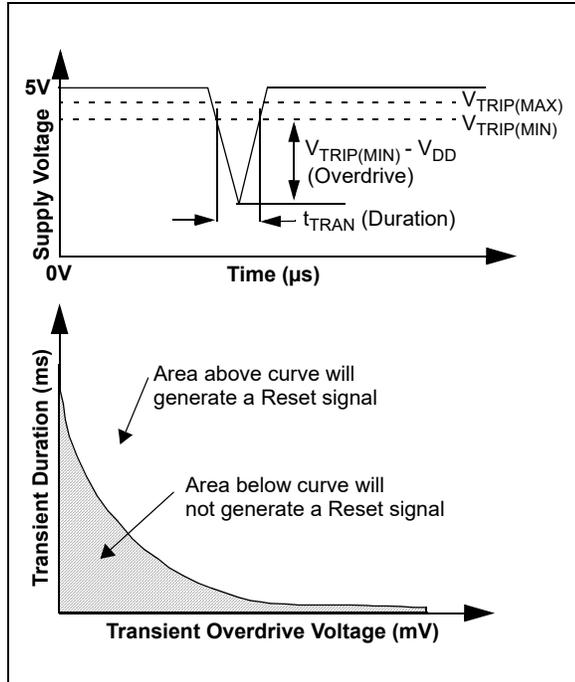
FIGURE 4-9: Example of Typical Transient Duration Waveform.
