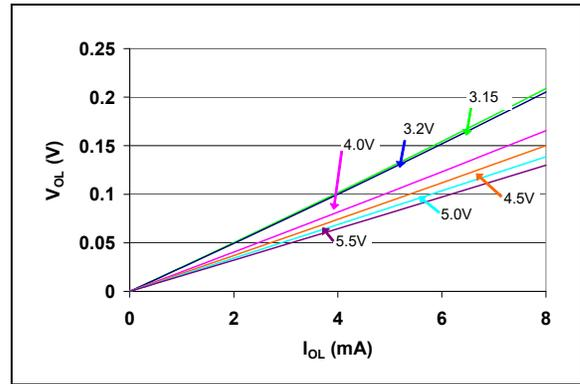
**FIGURE 2-17:**  $V_{OL}$  vs.  $I_{OL}$
