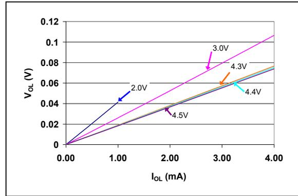
**FIGURE 2-16:**  $V_{OL}$  vs.  $I_{OL}$
