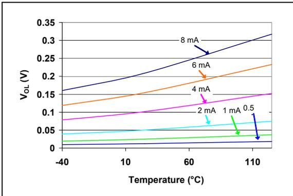
**FIGURE 2-20:**  $V_{OL}$  vs. Temperature
