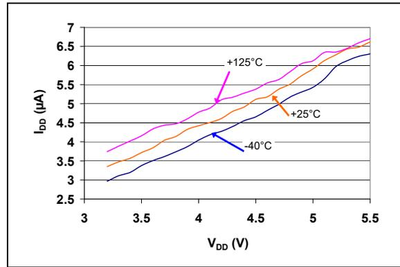
**FIGURE 2-11:**  $I_{DD}$  vs.  $V_{DD}$  (Reset Power-up Timer Active)
