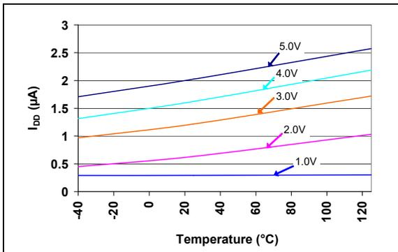
**FIGURE 2-2:**  $I_{DD}$  vs. Temperature (Reset Power-up Timer Inactive)
