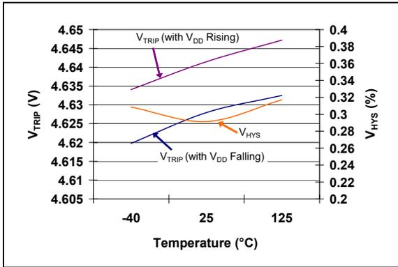
**FIGURE 2-13:**  $V_{TRIP}$  and  $V_{HYS}$  vs. Temperature
