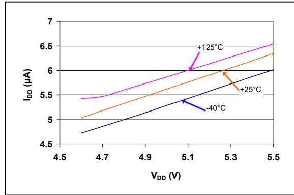
**FIGURE 2-10:**  $I_{DD}$  vs.  $V_{DD}$  (Reset Power-up Timer Active)
