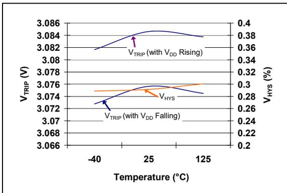
**FIGURE 2-14:**  $V_{TRIP}$  and  $V_{HYS}$  vs. Temperature
