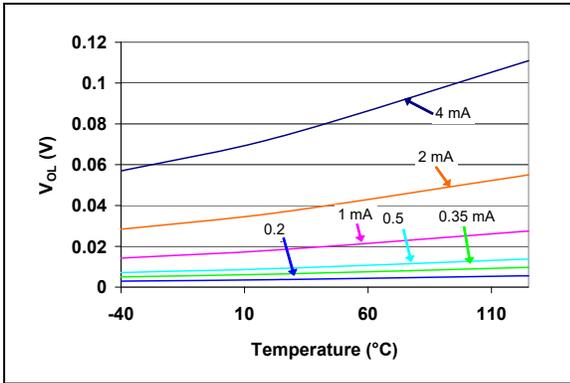
**FIGURE 2-19:**  $V_{OL}$  vs. Temperature
