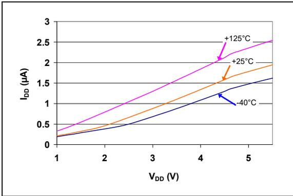
**FIGURE 2-7:**  $I_{DD}$  vs.  $V_{DD}$  (Reset Power-up Timer Inactive)
