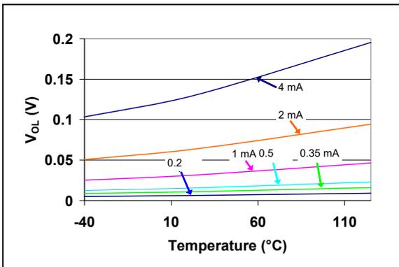
**FIGURE 2-21:**  $V_{OL}$  vs. Temperature
