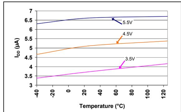
**FIGURE 2-5:**  $I_{DD}$  vs. Temperature (Reset Power-up Timer Active)
