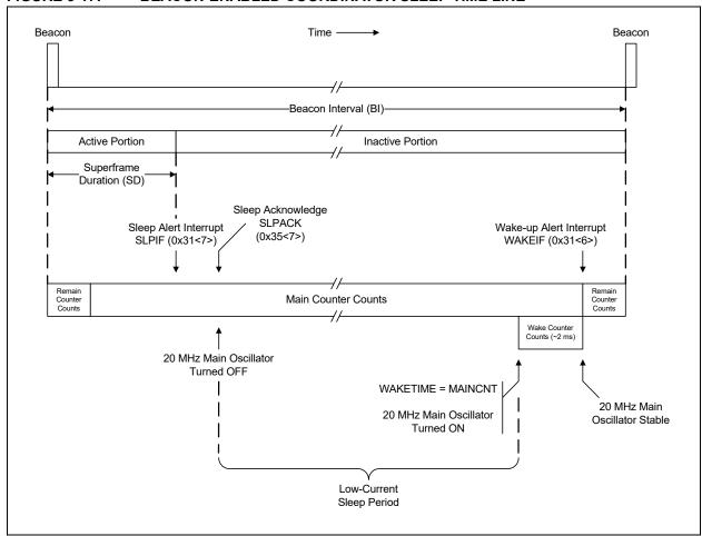
**Beacon-Enabled Device mode** – Figure 3-18 shows the Sleep time line for Beacon-Enabled Device mode. In this mode, the sum of the main and remain counters is the inactive period of the superframe. The MRF24J40 will time the inactive period as shown in Equation 3-4.
