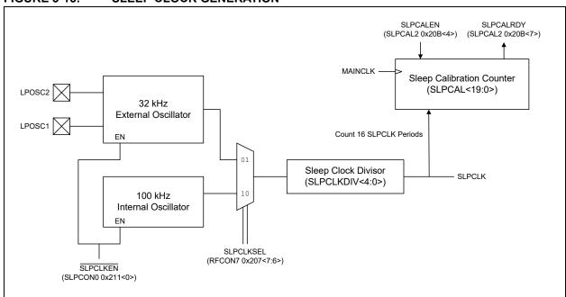
The 100 kHz internal oscillator requires no external components. However, it is not as accurate or stable as the 32 kHz external crystal oscillator. It is recommended that it be calibrated before use. See Section 3.15.1.2 "Sleep Clock Calibration" below for the Sleep clock calibration procedure.
