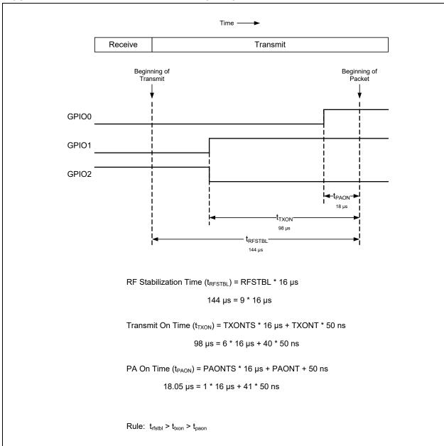
FIGURE 4-4: EXTERNAL PA/LNA TIMING DIAGRAM
