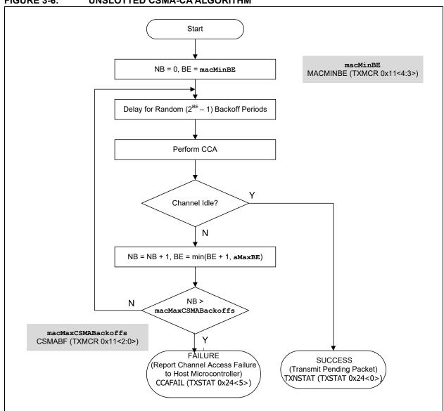
To configure the MRF24J40 for Unslotted CSMA-CA mode, clear SLOTTED (TXMCR 0x11[5]) bit = 0.
