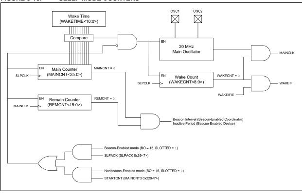
**Beacon-Enabled Coordinator mode** – Figure 3-17 shows the Sleep time line for Beacon-Enabled Coordinator mode. In this mode, the sum of the main and remain counters is the Beacon Interval (BI) of the superframe. The MRF24J40 will transmit a beacon packet as per Beacon Interval shown in Equation 3-3.
