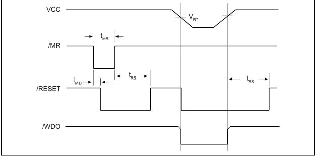
FIGURE 1-1: Reset Timing Diagram.
