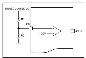
FIGURE 3-1: Power-Fail Comparator.
