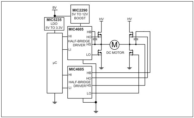
FIGURE 7-9: Full-Bridge DC Motor.
