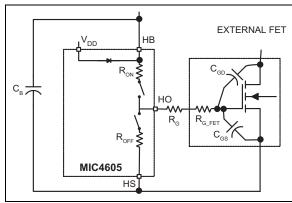
**FIGURE 7-1:** MIC4605 Driving an External MOSFET.
