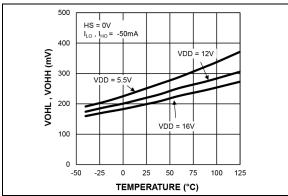
FIGURE 2-9: vs. Temperature.
