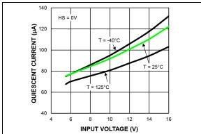
FIGURE 2-1: Quiescent Current vs. Input Voltage.
