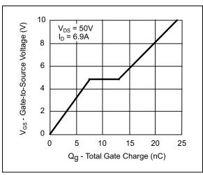
FIGURE 7-7: Typical Gate Charge vs. V<sub>GS</sub>.
