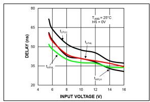
**FIGURE 2-4:** Propagation Delay vs. Input Voltage.
