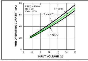
**FIGURE 2-3:** V<sub>HB</sub> Operating Current vs. Input Voltage.
