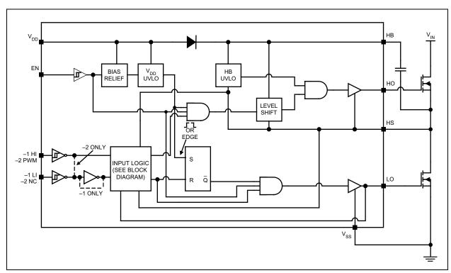
FIGURE 5-1: MIC4605 Top-Level Block Diagram.
