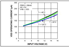
**FIGURE 2-2:** V<sub>DD</sub> Operating Current vs. Input Voltage.
