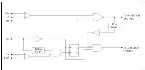
FIGURE 7-2: Adaptive Dead-Time Logic Diagram (PWM).
