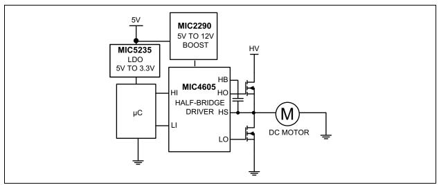
FIGURE 7-8: Half-Bridge DC Motor.
