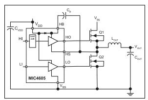
FIGURE 6-3: High-Side Driver and Bootstrap Circuit Block Diagram.
