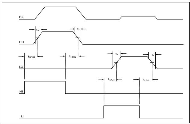
FIGURE 4-1: Separate Non-Overlapping LI/HI Input Mode (MIC4605-1).
