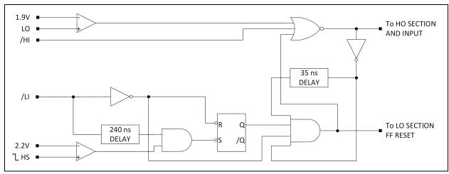
FIGURE 5-2: MIC4605-1 Cross-Conduction Lockout/PWM Input Logic Block Diagram.
