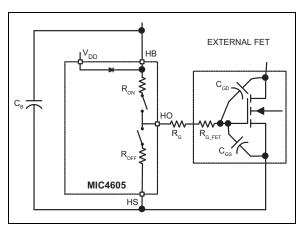
**FIGURE 7-6:** MIC4605 Driving an External MOSFET.
