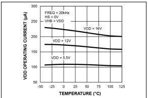
**FIGURE 2-6:**  $V_{DD}$  Operating Current vs. Temperature.
