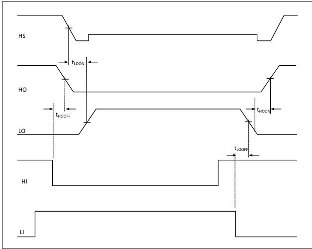
FIGURE 4-2: Separate Overlapping LI/HI Input Mode (MIC4605-1).
