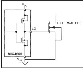
FIGURE 6-1: Low-Side Driver Block Diagram.
