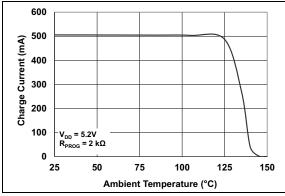
**FIGURE 2-15:** Charge Current  $(I_{OUT})$  vs. Junction Temperature  $(T_1)$ .
