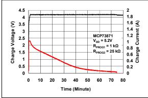
FIGURE 6-2: Typical Charge Profile (1000 mAh Battery).
