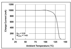
**FIGURE 2-14:** Charge Current ( $I_{OUT}$ ) vs. Junction Temperature ( $T_J$ ).
