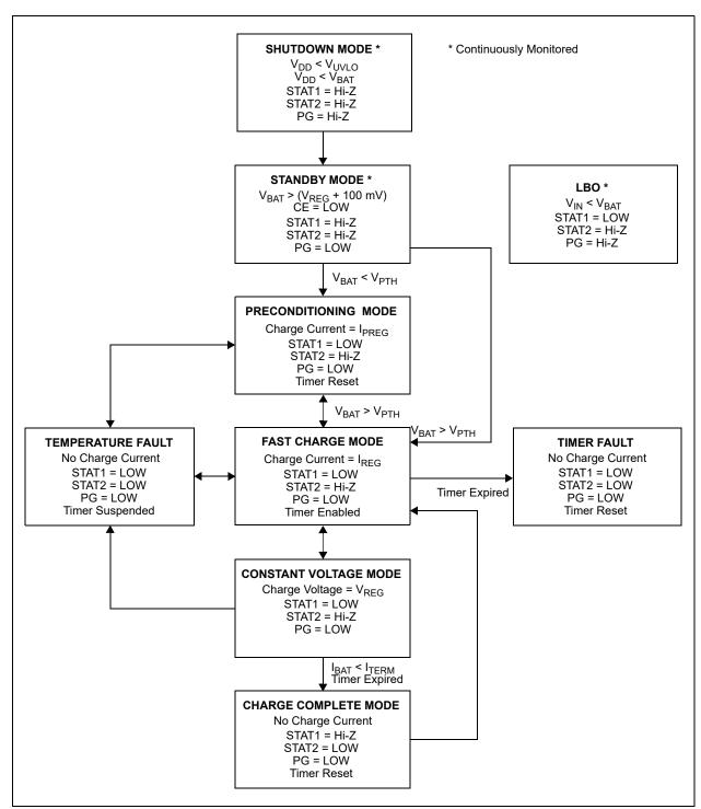
FIGURE 4-1: MCP73871 Device Flow Chart.
