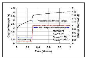
**FIGURE 2-29:** Typical Charge Profile in Preconditioning (1000 mAh Battery).
