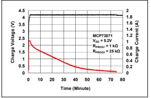
**FIGURE 2-28:** Complete Charge Cycle (1000 mAh Li-lon Battery).
