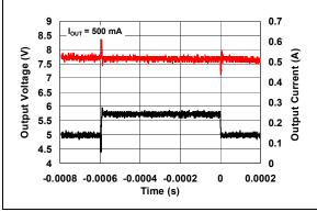
**FIGURE 2-21:** Line Transient Response.  $I_{OUT} = 500 \text{ mA}.$
