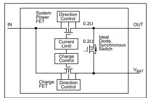
FIGURE 4-2: System Load Sharing Diagram.
