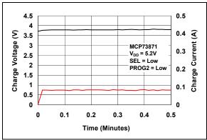
**FIGURE 2-26:** Start Charge Cycle (130 mAh Li-Ion Battery).
