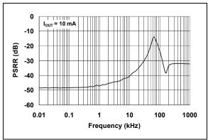
**FIGURE 2-19:** Power Supply Ripple Rejection (PSRR).
