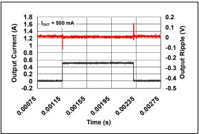
**FIGURE 2-23:** Load Transient Response.  $I_{OUT} = 500 \text{ mA}.$
