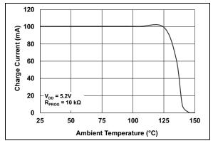
**FIGURE 2-16:** Charge Current  $(I_{OUT})$  vs. Junction Temperature  $(T_1)$ .
