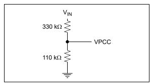
FIGURE 3-1: Voltage Divider Example.
