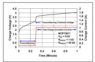
FIGURE 6-3: Typical Charge Profile in Preconditioning (1000 mAh Battery).
