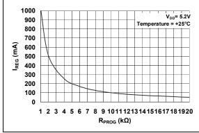
**FIGURE 2-3:** Charge Current ( $I_{OUT}$ ) vs. Programming Resistor ( $R_{PROG}$ ).
