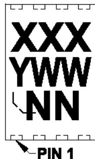
8-Lead TDFN (2x3x0.8 mm) (MCP6V77)
