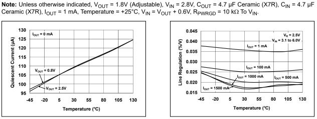
**FIGURE 2-16:** Line Regulation vs. Temperature (2.5V Fixed).
