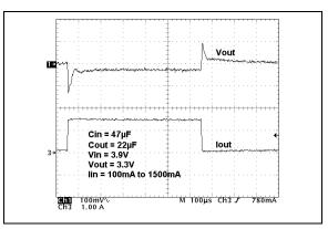
FIGURE 2-32: Dynamic Load Response (3.3V Fixed, 100 mA to 1500 mA).
