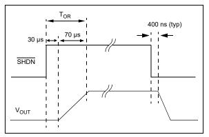
FIGURE 4-4: Shutdown Input Timing Diagram.
