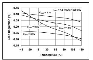
**FIGURE 2-5:** Load Regulation vs. Temperature (Adjustable Version).
