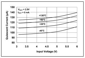
FIGURE 2-11: Quiescent Current vs. Input Voltage (2.5V Fixed).
