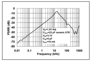
**FIGURE 2-24:** Power Supply Ripple Rejection (PSRR) vs. Frequency (V<sub>OUT</sub> = 1.2V Adj.).
