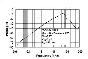
**FIGURE 2-25:** Power Supply Ripple Rejection (PSRR) vs. Frequency (V<sub>OUT</sub> = 3.3V Fixed).
