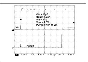
**FIGURE 2-29:** Power Good (PWRGD) Timing.
