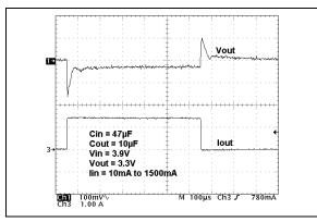
FIGURE 2-31: Dynamic Load Response (3.3V Fixed, 10 mA to 1500 mA).
