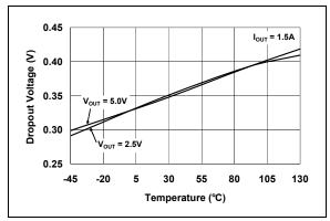
FIGURE 2-20: Dropout Voltage vs. Temperature.
