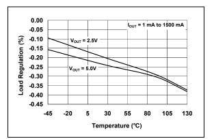
**FIGURE 2-18:** Load Regulation vs. Temperature ( $V_{OUT} \ge 2.5V$  Fixed).
