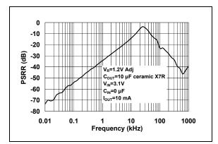
**FIGURE 2-23:** Power Supply Ripple Rejection (PSRR) vs. Frequency (V<sub>OUT</sub> = 1.2V Adj.).
