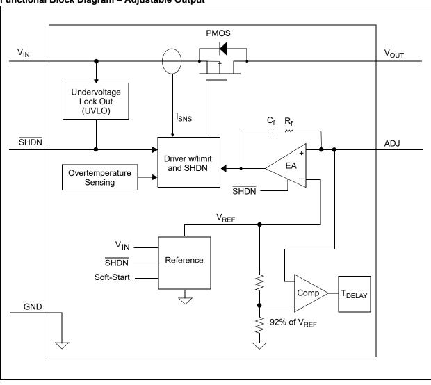
Functional Block Diagram – Adjustable Output
