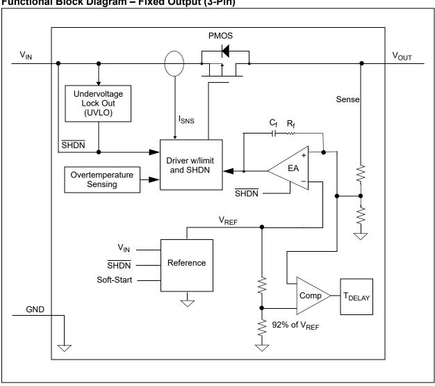
Functional Block Diagram – Fixed Output (3-Pin)
