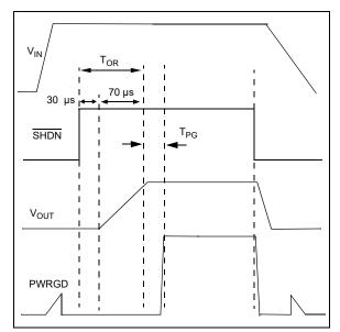
FIGURE 4-3: Power Good Timing from Shutdown.
