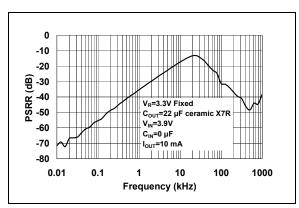
**FIGURE 2-26:** Power Supply Ripple Rejection (PSRR) vs. Frequency (V<sub>OUT</sub> = 3.3V Fixed).
