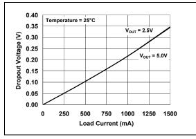
FIGURE 2-19: Dropout Voltage vs. Load Current.
