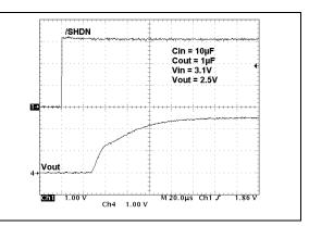
**FIGURE 2-28:** 2.5V (Adj.) Startup from Shutdown.
