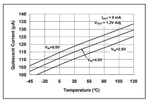
**FIGURE 2-3:** Quiescent Current vs. Junction Temperature (1.2V Adjustable).
