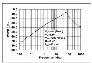
FIGURE 2-24: Power Supply Ripple Rejection (PSRR) vs. Frequency.
