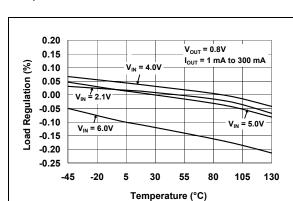
*FIGURE 2-17:* Load Regulation vs. Temperature.
