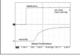
**FIGURE 2-26:** Startup from Shutdown (Adjustable Version).
