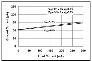
FIGURE 2-12: Ground Current vs. Load Current.
