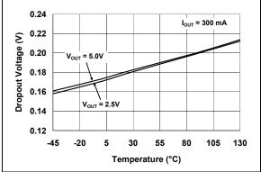
**FIGURE 2-20:** Dropout Voltage vs. Temperature.
