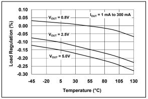
*FIGURE 2-18:* Load Regulation vs. Temperature.
