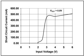
FIGURE 2-21: Input Voltage.
