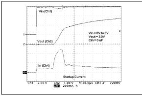
FIGURE 2-34: Startup Current.
