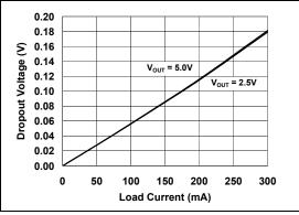
FIGURE 2-19: Dropout Voltage vs. Load Current.
