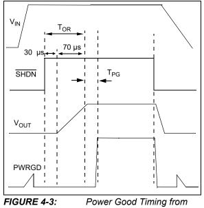
FIGURE 4-3: Power Good Timing from Shutdown.
