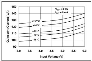
FIGURE 2-11: Quiescent Current vs. Input Voltage.
