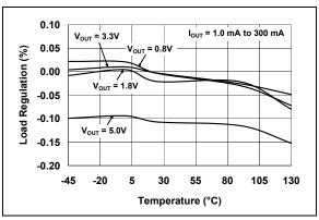
**FIGURE 2-5:** Load Regulation vs. Temperature (Adjustable Version).
