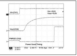
FIGURE 2-28: Power Good (PWRGD) Timing.
