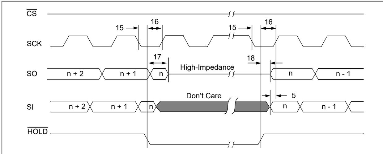
**FIGURE 1-2: SERIAL INPUT TIMING (SPI MODE)**
