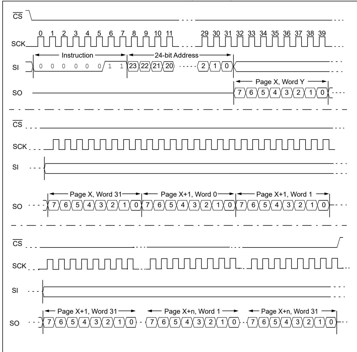
**FIGURE 2-6: SEQUENTIAL WRITE SEQUENCE (SPI MODE)**
