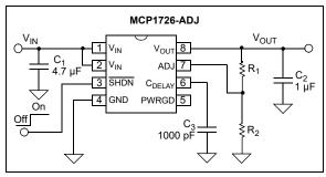
**FIGURE 4-1:** Typical Adjustable Output Voltage Application Circuit.
