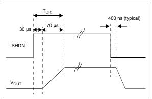
FIGURE 4-5: Shutdown Input Timing Diagram.
