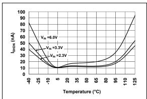
FIGURE 2-14: I<sub>SHDN</sub> vs. Temperature.
