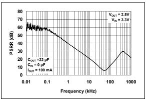
**FIGURE 2-26:** Power Supply Ripple Rejection (PSRR) vs. Frequency (V<sub>OUT</sub> = 2.5V Fixed).
