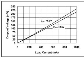
FIGURE 2-19: Dropout Voltage vs. Load Current.
