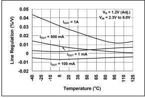
**FIGURE 2-4:** Line Regulation vs. Temperature (1.2V Adjustable).
