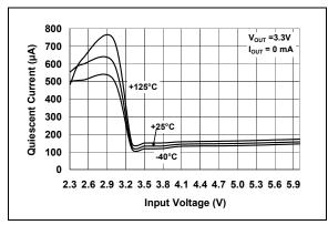
**FIGURE 2-11:** Quiescent Current vs. Input Voltage (3.3V Fixed).
