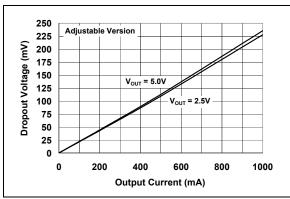
**FIGURE 2-7:** Dropout Voltage vs. Output Current (Adjustable Version).
