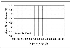
FIGURE 2-21: Short-Circuit Current vs. Input Voltage.
