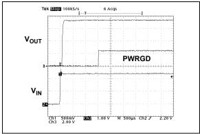
**FIGURE 2-29:** Power Good (PWRGD) Timing with C<sub>BYPASS</sub> of 1000 pF.
