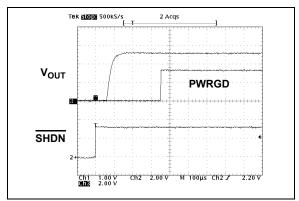
**FIGURE 2-28:** 2.5V (Adjustable) Start-Up from Shutdown.
