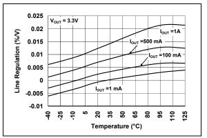
**FIGURE 2-16:** Line Regulation vs. Temperature (3.3V Fixed).
