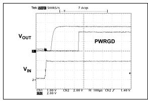
**FIGURE 2-27:** 2.5V (Adjustable) Start-Up from  $V_{IN}$ .
