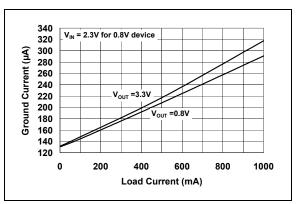
FIGURE 2-12: Ground Current vs. Load Current.
