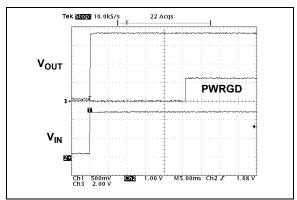
**FIGURE 2-30:** Power Good (PWRGD) Timing with  $C_{BYPASS}$  of 0.01  $\mu$ F.
