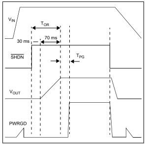
**FIGURE 4-3:** Power Good Timing from Shutdown.
