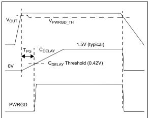
**FIGURE 4-4:** C<sub>DELAY</sub> and PWRGD Timing Diagram.
