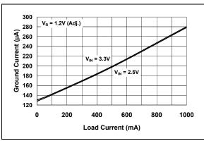
FIGURE 2-2: Ground Current vs. Load Current (1.2V Adjustable).
