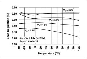
**FIGURE 2-5:** Load Regulation vs. Temperature.
