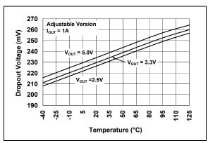
**FIGURE 2-8:** Dropout Voltage vs. Temperature (Adjustable Version).
