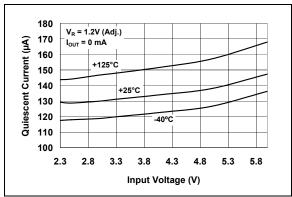
**FIGURE 2-1:** Quiescent Current vs. Input Voltage (1.2V Adjustable).
