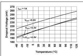
FIGURE 2-20: Dropout Voltage vs. Temperature.
