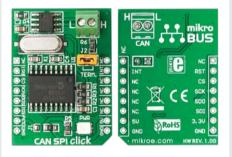
CAN SPI click 5V is an accessory board in **mikroBus**<sup>TM</sup> form factor. It is the best solution for adding CAN connectivity to your microcontroller with SPI interface. Board features **MCP2551** CAN transciever circuit which provides CAN serial communication physical layer in accordance with the ISO 11898 standard. It is designed for operation in especially-harsh environments, providing reliable solution. Board is designed to use 5V power supply only.
