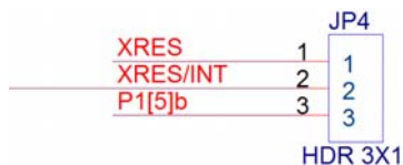
Figure 3-6. XRES/INT Selection Jumper
