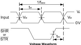
**Voltage Waveform Pulse Duration and Recovery Time**
