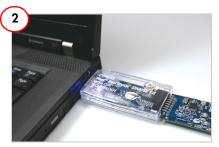
Program the RF Expansion board with RF\_12C\_Bridge.hex from the CD.
