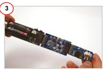
Connect the battery board, RF Expansion board, and the Weather Station board.
