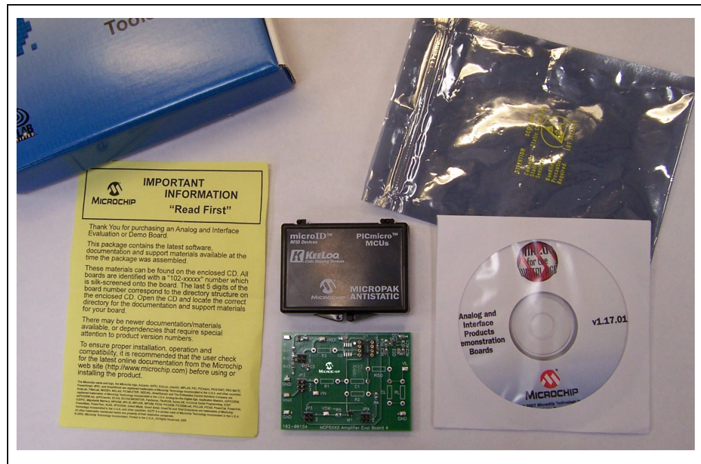
FIGURE 1-1: MCP6XXX Amplifier Evaluation Board 4 Kit.
