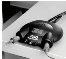
Figure 6: 3M™ Static Monitor 790 attached to equipment chassis
