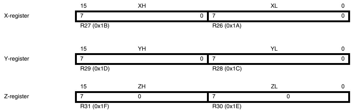
Figure 5-3. The X-, Y-, and Z-registers.
