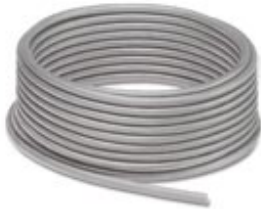
Cable ring, DeviceNet™/CANopen, 4-wire, shielded, PUR halogen-free, grey outer sheath, 2 x 0.34 mm²; 2 x 0.25 mm², cable length: 100 m
