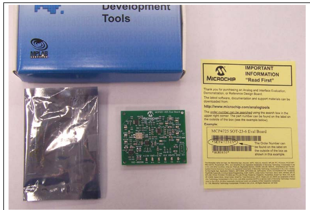
FIGURE 1-1: MCP651 Input Offset Evaluation Board Kit Contents.
