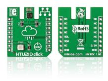
HTU21D click<sup>™</sup> carries a high-precision, easy-to-use relative humidity sensor with temperature output. The sensor is plug and play, requiring no calibration to use. The measurement range of HTU21D click<sup>™</sup> is from 0 to 100 percents of relative humidity, and -40 to +125 degrees of Celsius. The board communicates with the target microcontroller through mikroBUS<sup>™</sup> I2C lines: SCL and SDA (data). It uses a 3.3V power supply only.
