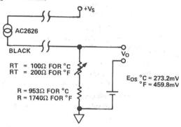
For most applications, a single point calibration is sufficient. With the probe at a known temperature, adjust  $R_{T}$  so that  $V_{O}$  corresponds to the known temperature.
