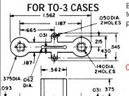
NYLON POWER TRANSIST OR MOUNT Barrier insulator, molded of type 6/6 natural colored nylon, functionally replaces up to six pieces of conventional insulation required with previous methods of mounting power transistors. Built-in barrier eliminates need for sleeving of connections.
