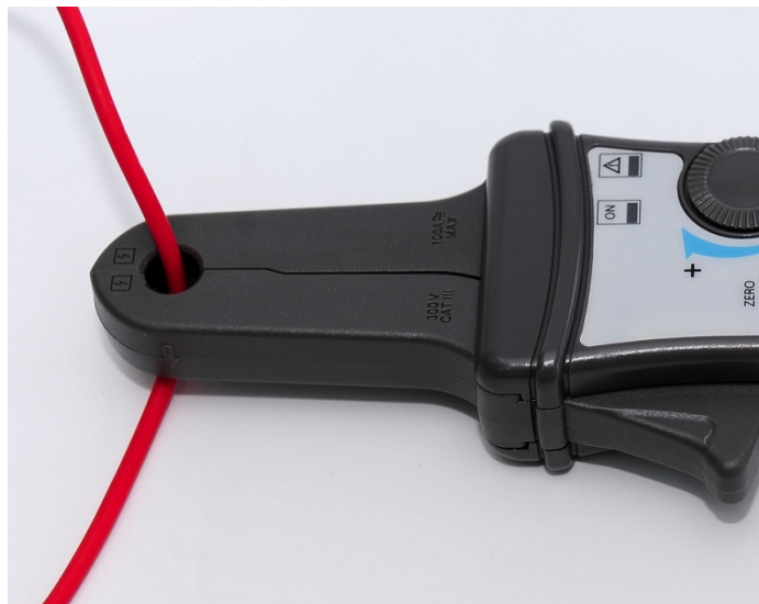
Figure 5: Connecting the CP62 current probe.
