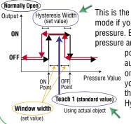
This is the ideal programming mode if you have a target pressure. Enter the target pressure and the ON and OFF
