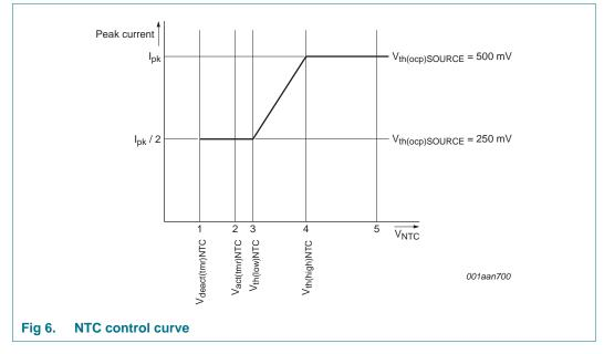
When the voltage on the NTC pin exceeds  $V_{th(high)NTC}$  (see Figure 6 (4)), the converter delivers nominal output current. When the voltage is lower than this level, the peak current is gradually reduced until  $V_{th(low)NTC}$  is reached (see Figure 6 (3)). The peak current is now half the peak current of nominal operation. When  $V_{act(tmr)NTC}$  is passed (see Figure 6 (2)) a timer starts to run to distinguish between the following situations:
