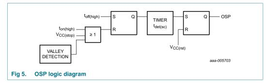
The value of  $t_{on(high)}$  depends on the capacitor connected to the TONMOD pin. An open or shorted TONMOD pin sets  $t_{on(high)}$  to 15 µs (see <u>Section 8.6</u> and <u>Table 6</u>).
