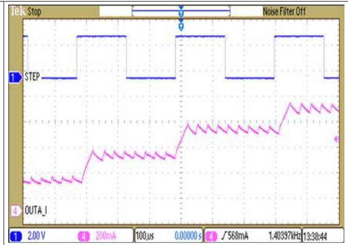
Figure 9. Microstepping Current (Phase A) vs STEP Input, Slow Decay on Increasing Steps
