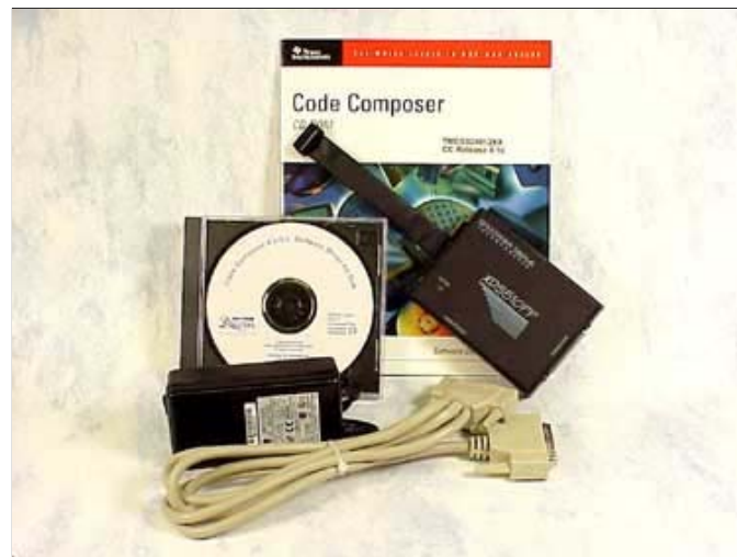
XDS510PP MPD Emulator with Code Composer for TMS320C3x/C4x
