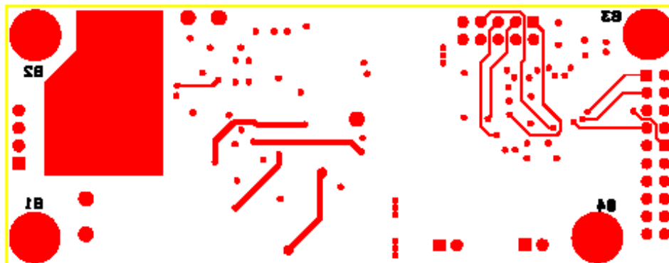
Figure 6: 73M1966B Demo Board Bottom Layer
