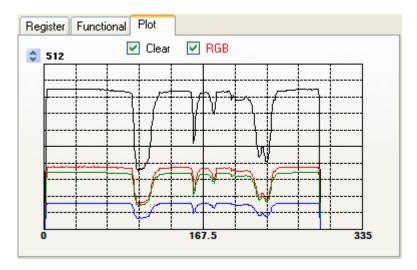
The graph shows all color outputs for the system. The X-axis plots 335 points then rolls over back to 0 on the graph. The Y-axis defaults to a range of 0 to 1024. The maximum Y value can be adjusted by clicking on the up and down buttons beside the range value. This maximum value may be set to any power of two starting at 64, up through 32768. The checkboxes above the graph control which values will be included on the graph.
