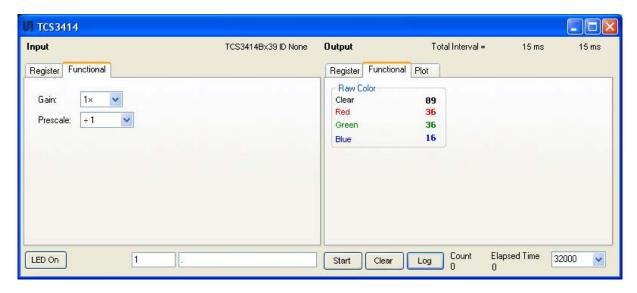
This window has inputs organized on the left, and outputs organized on the right. Values for register variables may be set using multiple techniques. The Functional tab is commonly used to quickly evaluate the device with nominal settings. The Input Register tab allows the register settings to be changed, and the Output Register tab allows registers to be viewed.
