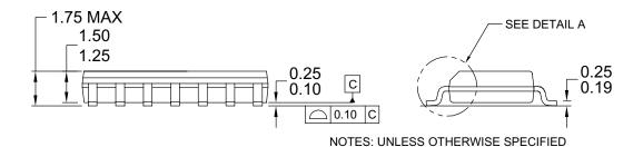
A) THIS PACKAGE CONFORMS TO JEDEC MS-012, VARIATION AB, ISSUE C, B) ALL DIMENSIONS ARE IN MILLIMETERS. C) DIMENSIONS DO NOT INCLUDE MOLD
