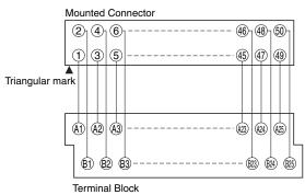
Note: For all models, the odd-numbered pins on the Connector correspond to row A on the terminal block and the even-numbered pins on the Connector correspond to row B on the terminal block.
