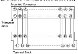
Note: For all models, the odd-numbered pins on the Connector correspond to row A on the terminal block and the even-numbered pins on the Connector correspond to row B on the terminal block.
