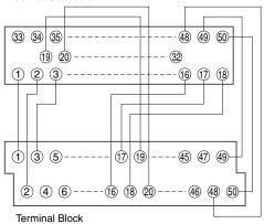
Note: Connector pin numbers correspond 1-to-1 to terminal block numbers on all models.
