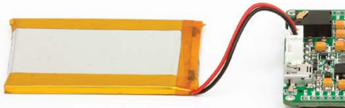
Figure 1-2: Connecting Li-Polymer battery
