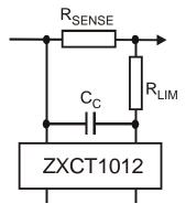
If large reverse currents are expected then the resistor, RLIM, will provide protection from exceeding absolute maximum ratings.
