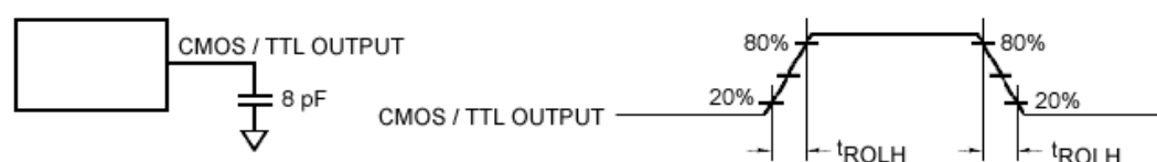
Figure 9. Receiver LVTTL/CMOS Output Load and Transition Times
