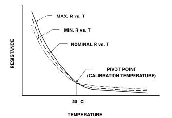
Point match resistance tolerances at temperatures other than  $25\ ^{\circ}\text{C}$  are not the same as the calibration temperature. This difference is presented in Figure 2.
