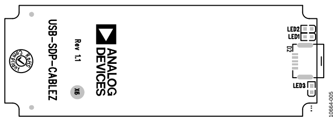
Figure 5. USB-SDP-CABLEZ Board LEDs
