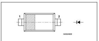
Marking code: A7 The marking bar indicates the cathode.
