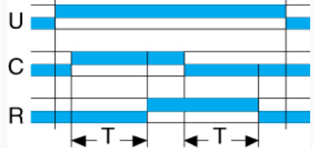
Function Ac - 1 relay output
