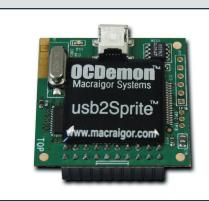
The usb<sup>2</sup>Sprite is a self-powered, cable-less, miniaturized (2.25 in<sup>2</sup>) version of our usb<sup>2</sup>Demon that plugs directly into a board's JTAG/BDM header providing "built-in" debug connectivity. To the user the usb<sup>2</sup>Sprite looks like a USB mini connector sitting on top of the board's JTAG/BDM header. Problems caused by customer installation errors, JTAG cable noise, parallel port incompatibility, and the need for an external power supply are eliminated.
