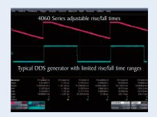
Capable of setting edge times within a large range, the 4060 Series can generate pulses with minimum rise/fall times of 6 ns and maximum rise/fall times of 6 seconds...
