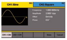
Save time with the 4060 Series' two independent channels to output synchronous signals. With a push of a button, all waveform parameters can be quickly copied between channels to set up identical output signals. Phase between channels can also be adjusted from the front panel.
