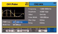
These instruments are capable of many different types of modulation for various applications. Modulate your waveforms with AM, DSB-AM, FM, PM, ASK, FSK, and PWM modulation schemes.
