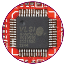
Figure 9-1: On-board VS1053 MP3 codec
