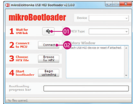
Figure 3-2: USB HID mikroBootloader window
