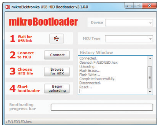
Figure 3-8: mikroBootloader ready to use
