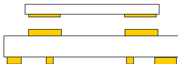
Figure 20. Correct PCB Top Metal Pattern Under Package
