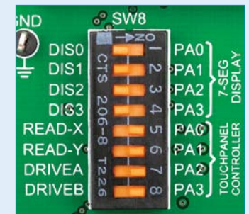
Figure 12-5: Turn on switches 5 through 8 on SW8 to enable Touch panel controller
