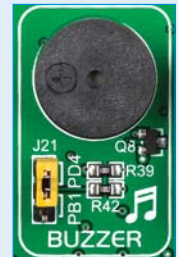
Figure 18-2: Use jumper J21 to connect Piezo buzzer on PB1 or PD4 pin
