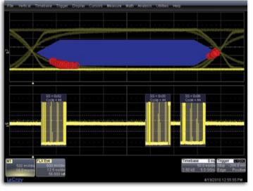
Gain valuable insight into your FlexRay communications channel by viewing eye diagrams, physical layer measurements and decoded protocol data at one time.
