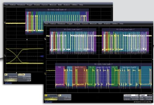
Trigger on Static or Dynamic Slot IDs and FlexRay Symbols, apply a color-coded, easy-tounderstand decode over your FlexRay signal, perform automatic eye diagram mask testing and make physical layer timing measurements.
