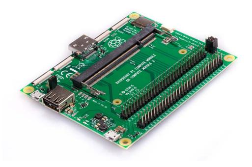
The Compute Module IO Board V3 is a development kit for those who wish to make use of the Raspberry Pi in a more flexible form factor, intended for industrial applications. The IO Board V3 is made for developing with CM3, CM3L, and CM1. This kit replaced the original Compute Module IO Board in January 2017.
