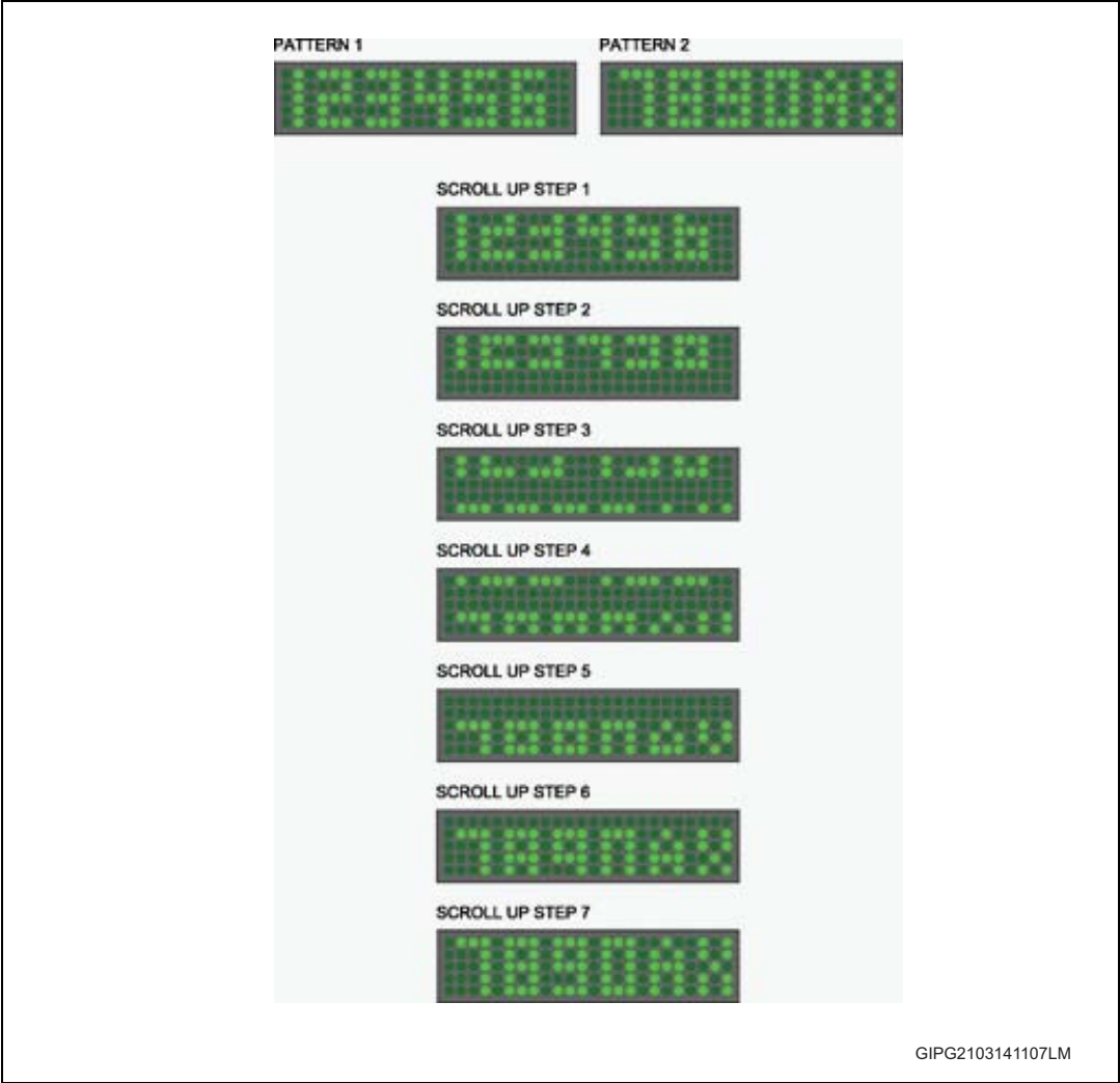
Figure 14. Example of scroll with 2 inserted blank rows (BRCEN=1, DISP 01 → 10)
