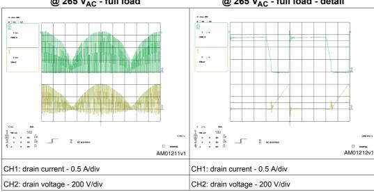
*Figure 14* shows the measurement at the maximum drain voltage of 265  $V_{AC}$  and max load. In this worst-case condition, the peak drain voltage is 640  $V_{PK}$ , assuring a good margin with respect to the MOSFET BV<sub>DSS</sub> and contributing strongly to the reliability and low failure rate of the design.
