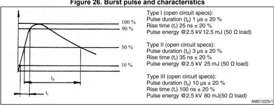
Figure 26. Burst pulse and characteristics
