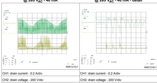
Figure 18. EVL6562A-35WFLB  $V_{DS}$  and  $I_{D}$  Figure 19. EVL6562A-35WFLB  $V_{DS}$  and  $I_{D}$  @ 265  $V_{AC}$  - 40 mA - detail
