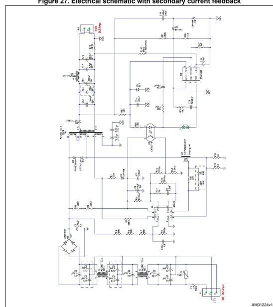
Figure 27. Electrical schematic with secondary current feedback
