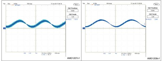
In *Figure 10* and *Figure 11* the output voltage ripple at twice the input mains frequency is measured. As shown it is less than 0.4 V peak-to-peak, which is ideal for LED or lighting applications. High frequency noise, including spikes, is significantly reduced as well.
