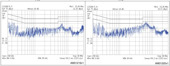
Figure 24. 230 V<sub>AC</sub> and full load - phase Figure 25. 230 V<sub>AC</sub> and full load - neutral
