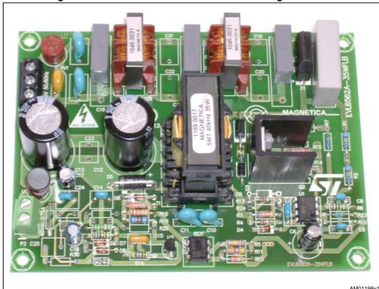
Figure 1. EVL6562A-35WFLB evaluation board using the L6562A
