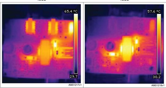
Table 2. Measured temperature @ 90  $V_{AC}$  and 265  $V_{AC}$  - full load
